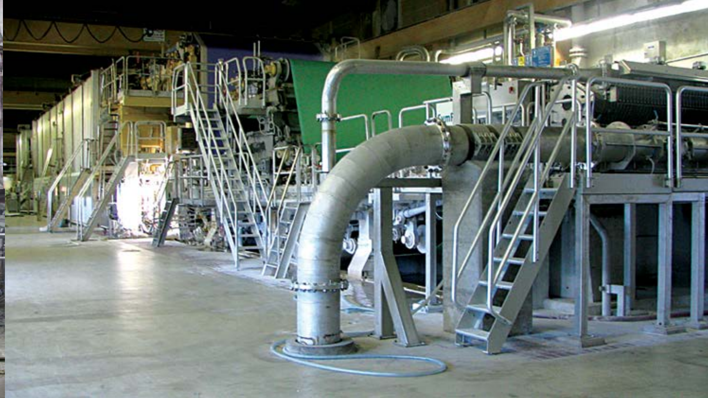
Paper machine after the 2006 upgrade – new headbox and new top wire
